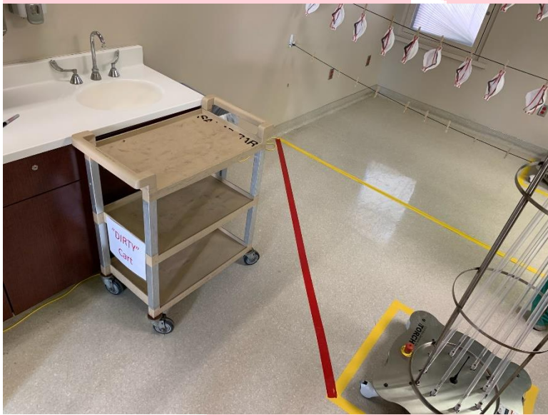
Figure 10 – Do not block UVGI arc from light to respirators.
